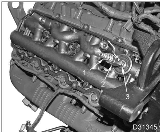
Figure 10 Compressed air supply with valve cover off
