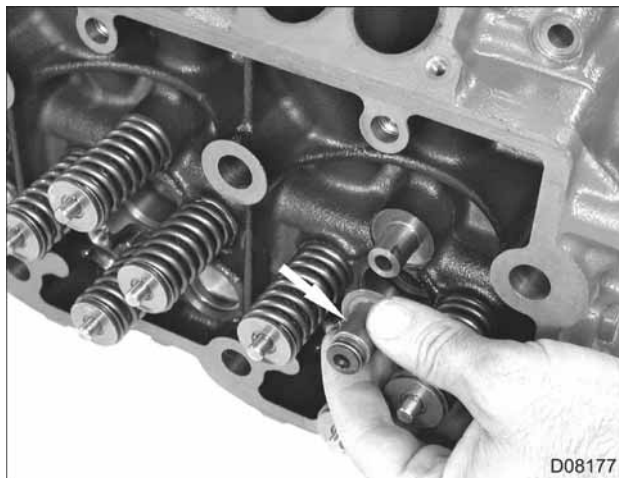
Figure 174 Valve stem oil seal
