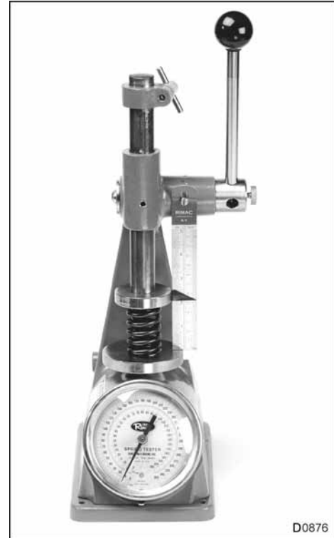
Figure 205 Measurement of valve spring free length
