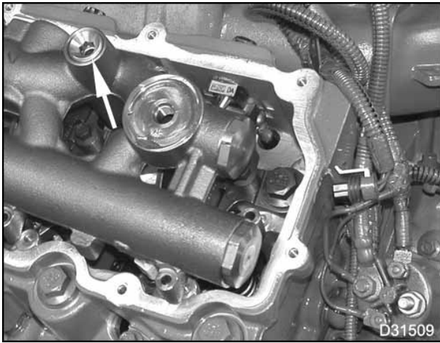
Figure 265 Crankcase-to-head tube plug (hex head)
