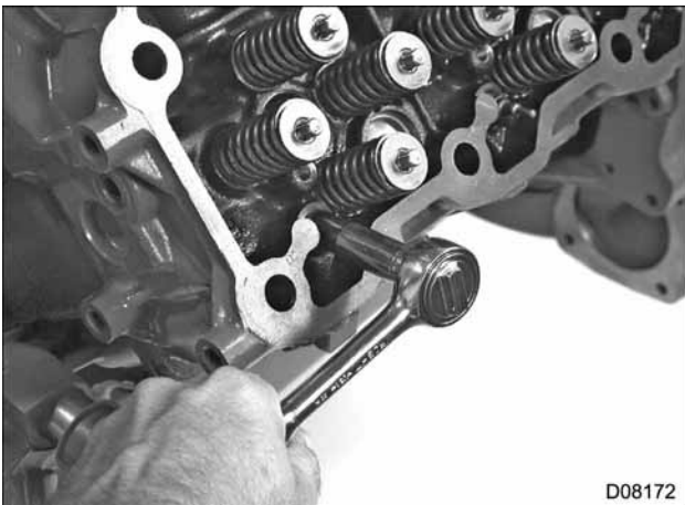
Figure 163 Glow plug removal
