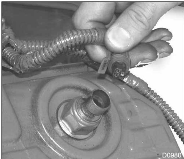
Figure 135 Electrical connector removed from ICP sensor
