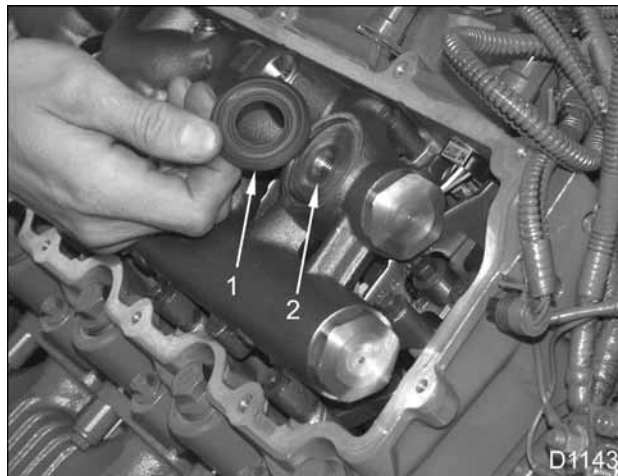
Figure 137 Valve cover seal ring for ICP sensor
