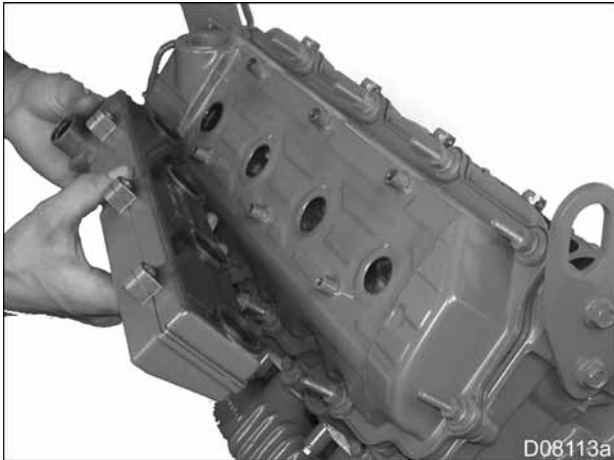
Figure 143 Breather housing
