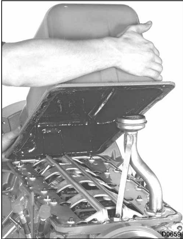
Figure 315 Lower oil pan
