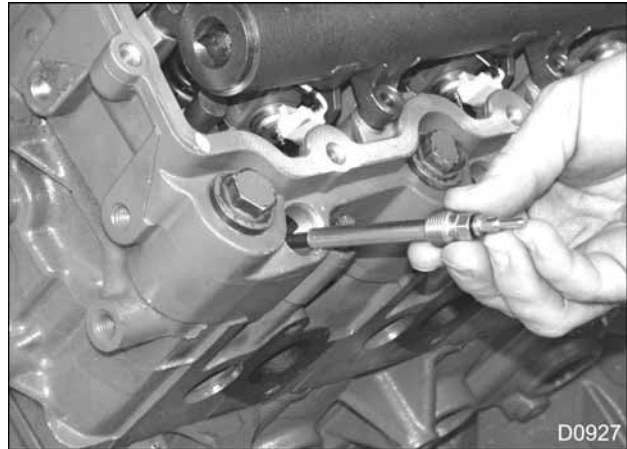
Figure 266 Installation of glow plug
