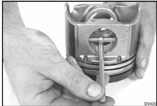
Figure 334 Inside diameter measurement of piston pin bore
