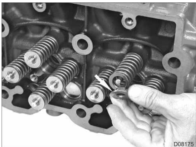
Figure 171 Valve spring retainer
