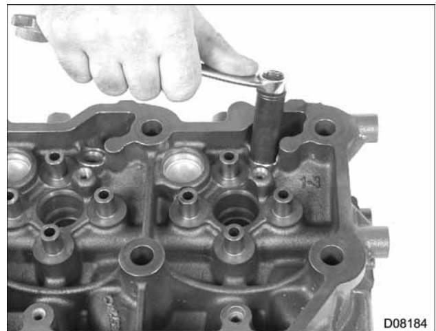
Figure 183 Removal of glow plug sleeve
