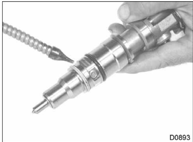
Figure 252 Lubrication of fuel injector O-rings
