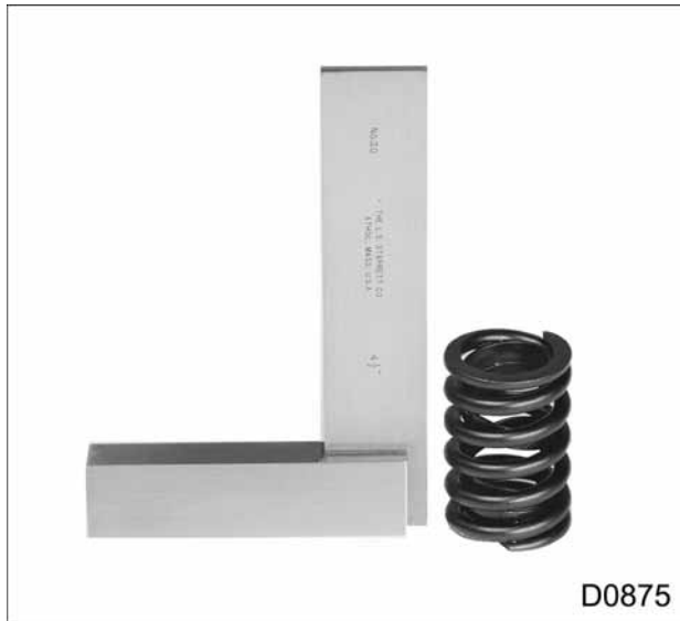
Figure 204 Flatness check of valve spring
