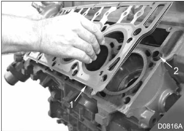
Figure 233 Installation of cylinder head gasket
