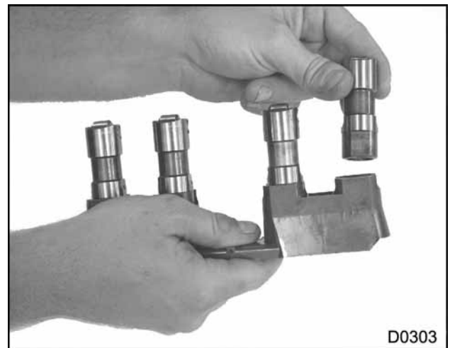
Figure 168 Cam follower removal from roller follower guide
