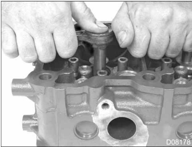
Figure 176 Fuel injector sleeve tapped
