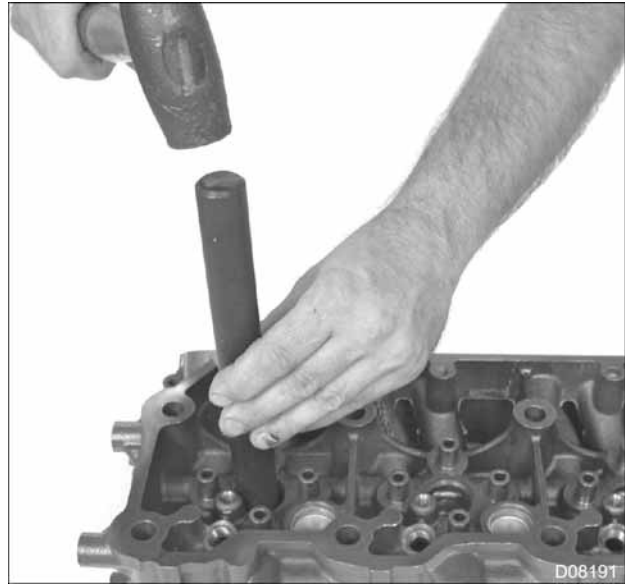
Figure 212 Installation of fuel injector sleeve into bore
