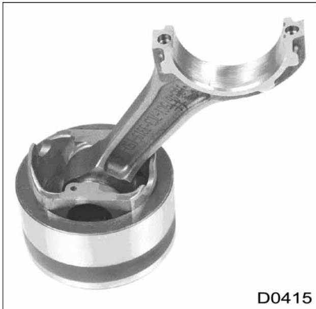
Figure 343 Piston installed in piston cope
