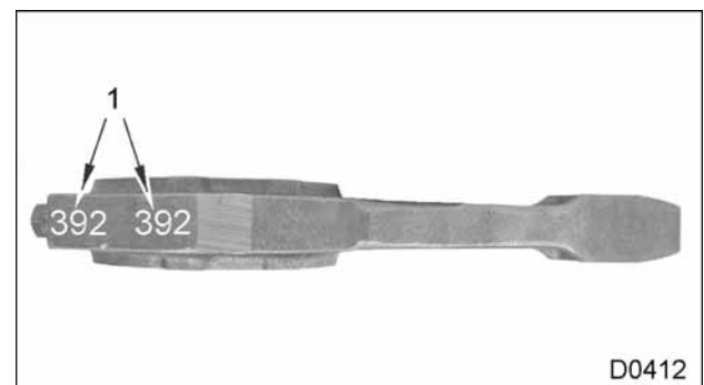
Figure 321 Cap and rod numbers
