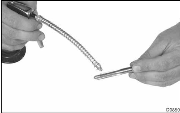
Figure 180 Glow plug sleeve remover (Thread tap)
