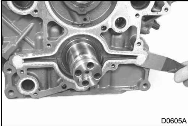
Figure 288 Sealant between crankcase and lower crankcase joint
