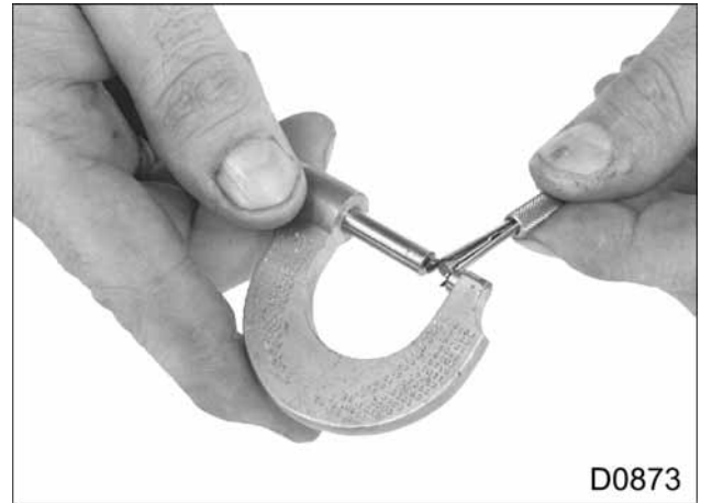
Figure 201 Measurement of Small Hole Gauge (valve guide ID)
