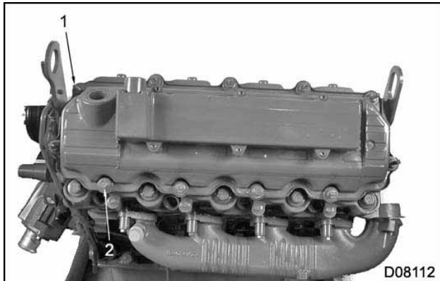
Figure 271 Valve cover mounting bolts and studs
