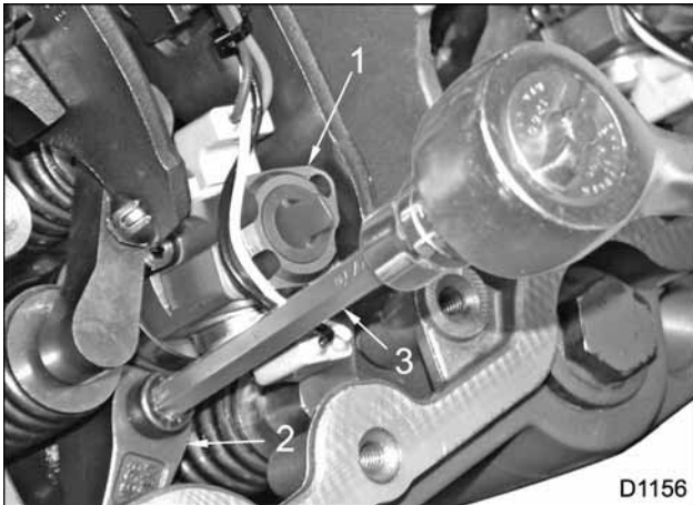
Figure 257 Fuel Injector Hold Down Wrench installed
