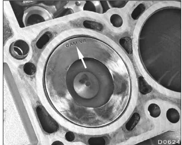
Figure 342 CAM V8 stamp on piston
