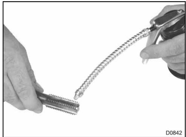
Figure 175 Lubrication of Injector Sleeve Remover (Thread tap)
