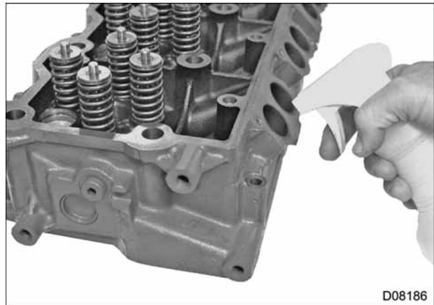
Figure 198 Intake and exhaust ports sprayed with mineral spirits
