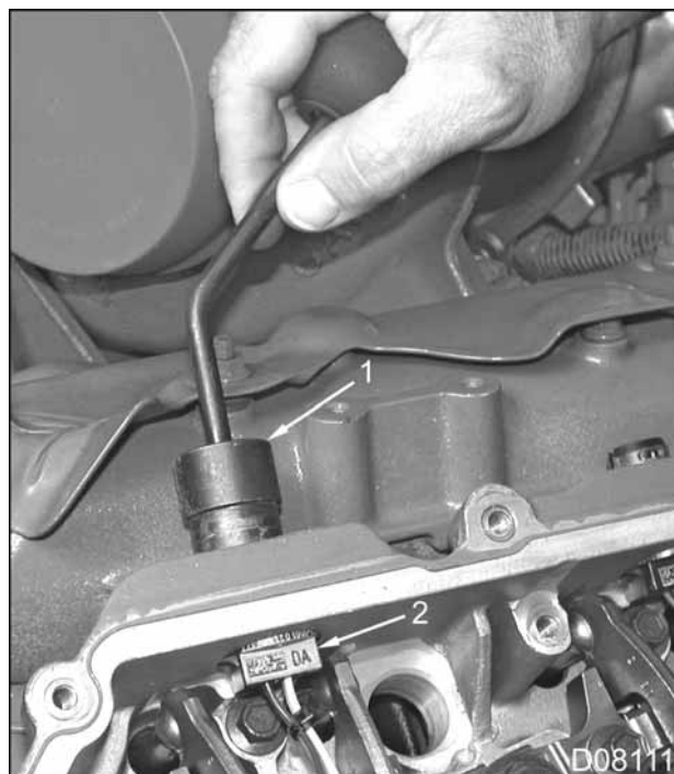
Figure 152 Injector connector removal
