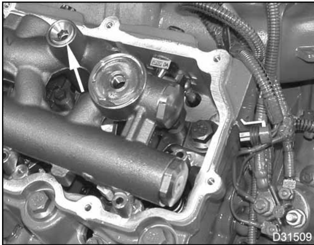
Figure 146 Crankcase-to-head tube plug
