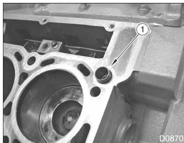
Figure 232 Cylinder head spring dowel pin in crankcase (typical)
