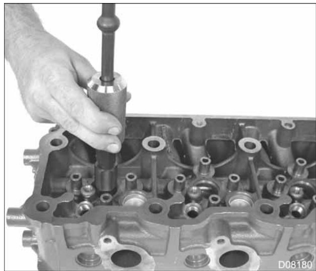
Figure 178 Slide hammer
