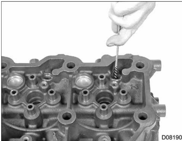
Figure 210 Glow plug bore
