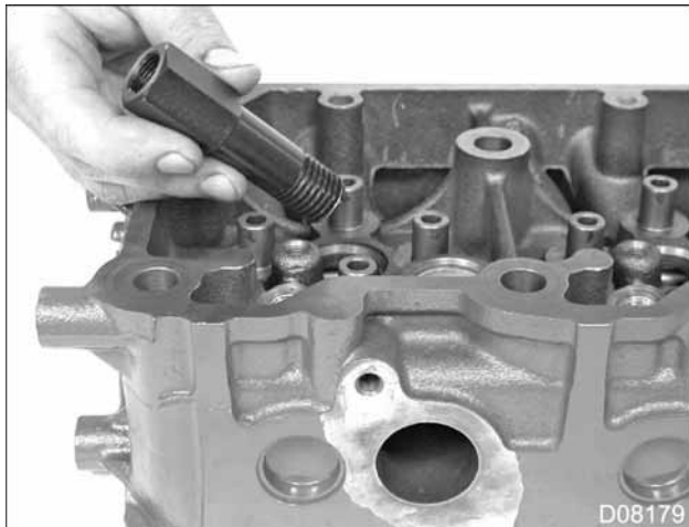
Figure 177 Injector Sleeve Remover (Slide hammer adapter)
