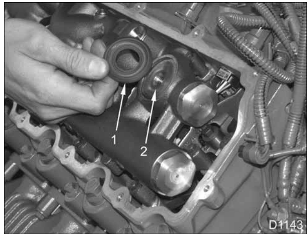
Figure 144 Valve Cover Seal Ring for ICP Sensor
