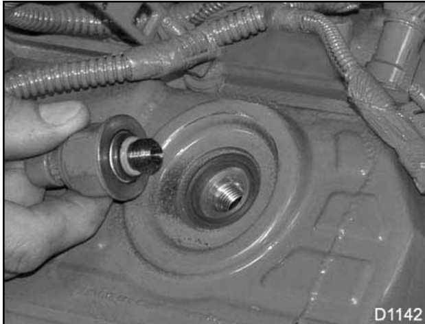
Figure 268 ICP Sensor and O-ring
