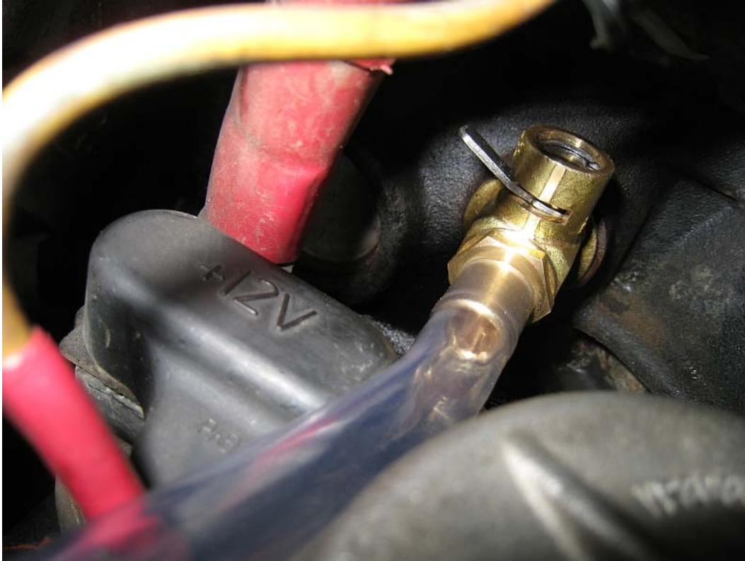
Fig 8.2 Fumoto valve inserted in passengers side drain plug with optional drain hose.
