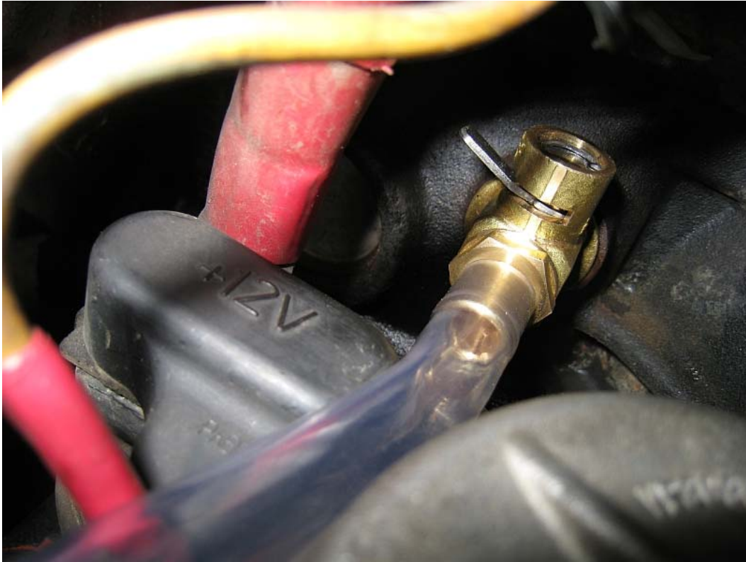
Fig 5.2.2 location of passenger side drain plug shown with Fumoto valve installed.
