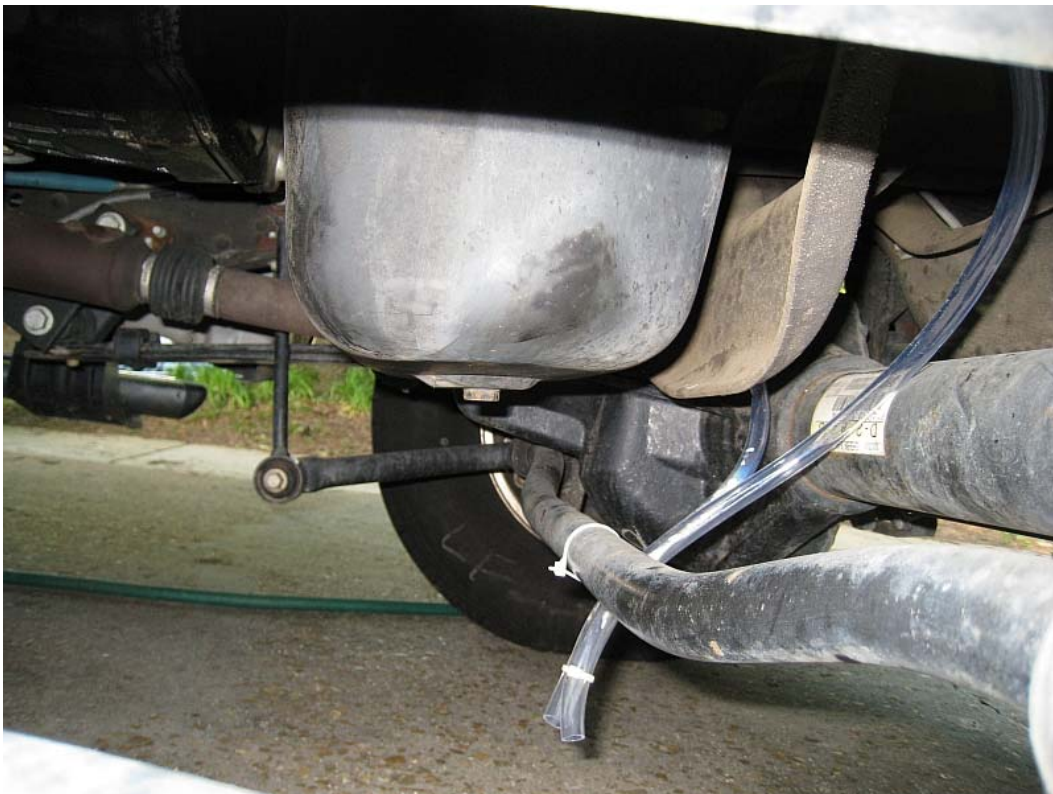
Fig 8.3 Drain hoses routed to underside of vehicle for collection
